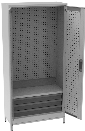
MPC-04 W900 D400 H1925 mm GI Shelves -90 kg UDL 100mm Drawer -3 Nos ( 35 kg UDL ) Effective Height - 70mm
